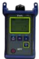
MFP Multi-Fiber Power Meter
