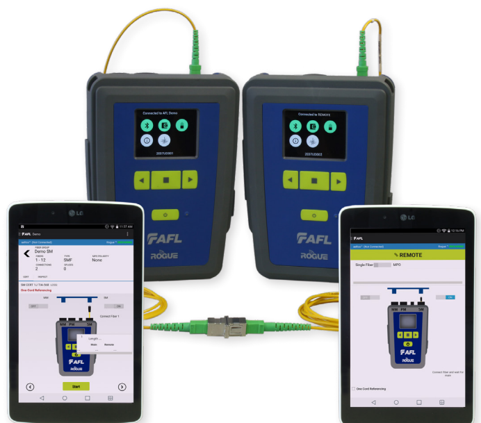
ROGUE OLTS Certifier kit with cB1 Bases and required smart devices (optional purchase)
