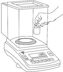
4. When prompted, load a calibration weight equal to the weight displayed on the screen. (Calibration weight varies by model).
