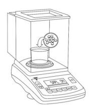
6. The scale will flash "FI LL" and then display the sample size (**Example**: 10 pcs) indicating to begin filling the remainder of the count. Begin to pour the pills into the container.
