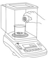
9. After the container with the counted pieces has been removed, the command "---, <code>[DUnt Fln/5H, LDUnt Press C"</code> will appear on the display sequentially. Press the "CLR" key to begin a new count.
