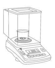
7. The display will now indicate the number of pieces placed in the container. Stop filling when the desired count has been reached.
