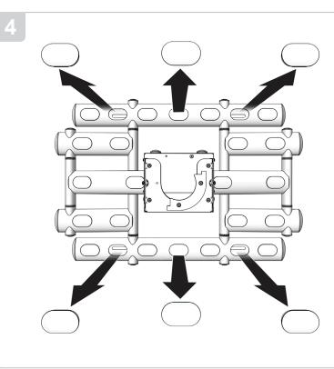
Take the mounting template supplied insure the template is centered and level at the desired height on the mounting surface. Mark the mounting hole (six recommended) three on top and three on bottom.
