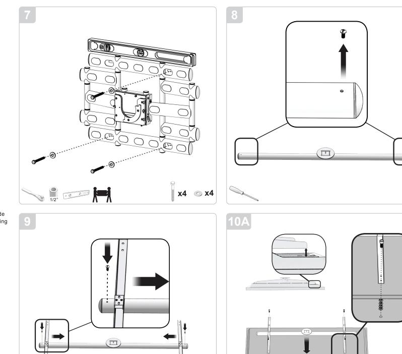
Remove the two security screws from the right and left side of the mounting bracket crossbar and slide the two mounting brackets inside the left and right side security screw hole and reinstall the two security screws.
