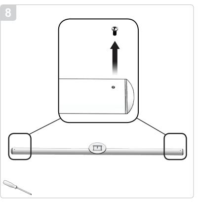
Remove the two security screws from the right and left side of the mounting bracket crossbar and slide the two mounting brackets inside the left and right side security screw hole and reinstall the two security screws.
