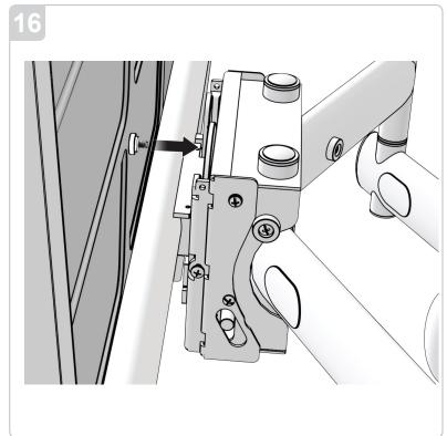
Add. Once all mounting points and level of the display have been confirmed the plastic covers may be installed to provide a clean look to the in stalled display and mount.
