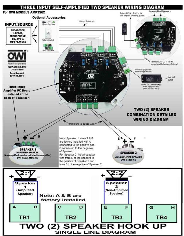
Filename: AMP3IC6 3 Input Detailed Wiring Diagram 2 SPEAKER 10/24/12
