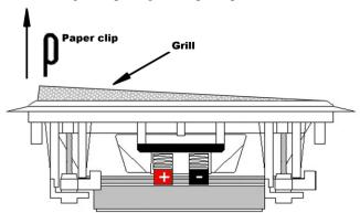
Be sure to position the four Mounting Tabs on your OWI speaker inward, then insert the four screws (supplied) from the front of the speaker into the screw opening.
