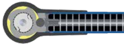
Working principle of the Gedore Torque Slipping Wrenches
