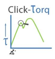
In Click-Torque mode, the first peak reading will remain on the OLED display when the load is removed as long as the torque loaded is above the 10% of maximum capacity threshold. This mode is used in conjunction with mechanical clicker type wrenches. The wrenches are generally calibrated to the click-torque value. The user has the option to store the reading in memory. If storage of the reading is not required, the user may continue to the next measuring task.
