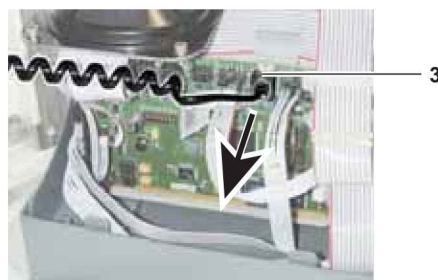
Fig. 3: Disconnection of the control panel cable
