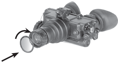
Figure 2-5. Installation of the Light Interference Filter
