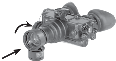
Figure 2-4. Installation of Compass
