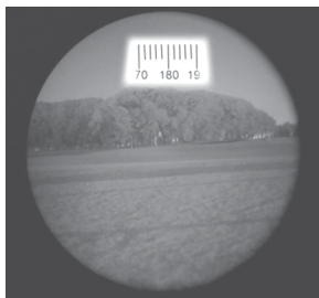
Figure 2-12. View Through Installed Compass
