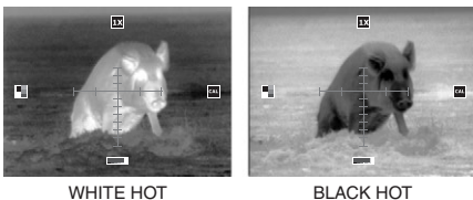
FIGURE 3.12. DISPLAY POLARITY MODES
