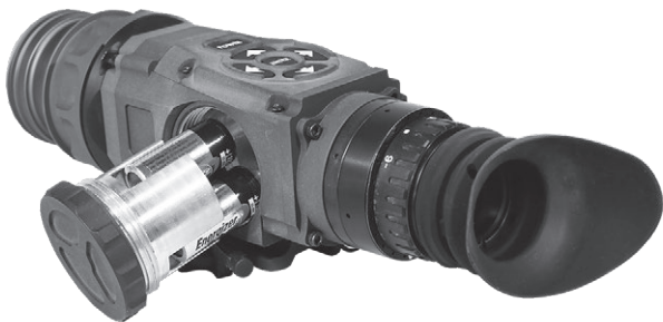
FIGURE 2.2. INSTALL BATTERY MODULE
