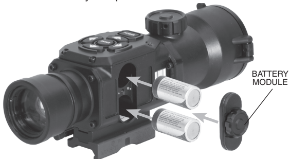
FIGURE 2.1. LOADING BATTERY MODULE
