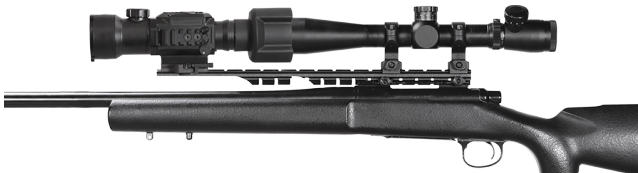
FIGURE 2.5. TICO WITH LEUPOLD DAY SCOPE ON LONG RAIL
