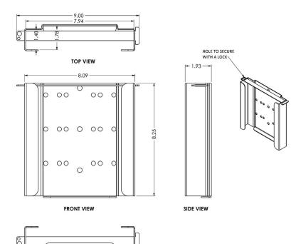
The **BKT-MCM** Mac Mini bracket allows you to easily install your Mac Mini Apple small desktop computer or other similar devices. Its design securely attaches onto our products or it can be wall mounted. Constructed from durable steel and powder coated black. Padlock not included.
