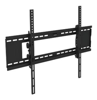
The wall mount WM-6090 supports 55" to 90" flatscreen TV's weighing up to 220 lbs. Vesa max 900 x 500mm. Tilt range is -15 to +15 degrees. Generic wall mounts are not manufactured by us and are provided for your convenience. We tested for strength and compatibility with our accessories.
