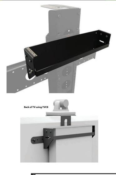
The **PM-2RU** provides the ability to rack mount codecs and CPU's to PM-Series Spines, back of TV's (using TVCB), and wall mounting (16" spaced mounting holes). It features 2 rack units with one reinforcement strip to hold electronics in place during transportation.
