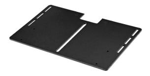
The **PM-CMP** was designed as an add-on for the standard cam tongue on PM series mounts and XLD mount. When a set mounted codec is required, the **PM-CMP** features a large surface designed to fit most of today's codecs and wider cameras such as the \*EagleEye™. Slots for mounting straps and a long adjustable slot for a 1/4-20 bolt. Includes mounting hardware.
