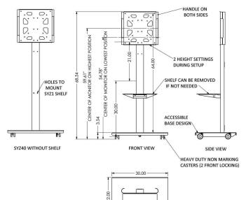
The **SYZ40-W/B** modern mobile stand, features a base that allow easy access and it can be easily rolled from location to location.
