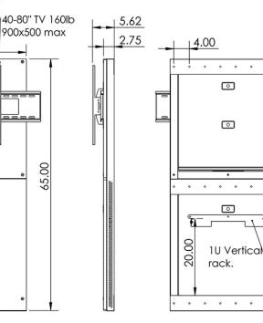
**TP200-WM** wall offset stand for single monitor applications. A wall mounted metal frame with ventilation, 1U rack and cable management for keeping your install simple and external to wall. Standard color is black. The TP200-WM accommodates 40"-80" displays (160 lbs max). See your monitor manufacturers website for installation guide or spec to confirm mounting hole locations. Max mount hole location is 900mm wide X 500mm high.
