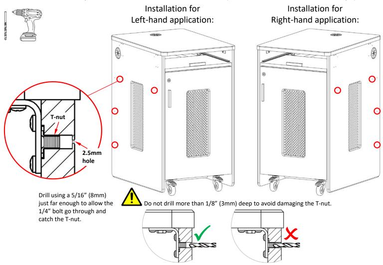
After drilling, install corner braces with bolts needed to attach the Skirt and Top panels as shown below. Do Not overtighten the bolts, all parts will be reinforced with screws at the end of assembly.
