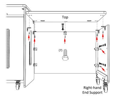
Once all parts are in place and bolts are tightened, drive in the 5/8" screws provided to all corner braces to reinforce.
