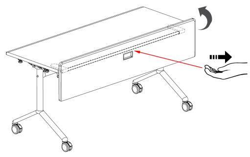
Pressing down the latch on both brackets will fold the modesty panel. To unfold the table, reverse the procedure, both folding mechanism and the brackets will self-lock into the open position.
