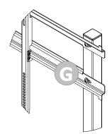
Place the Support Display mount **I-J** at the top between the body **A,** using 5/16" x 3/4" Phillips screw head and 5/16" washer (4x) **G.**
