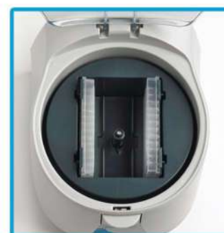
During centrifugation (horizontal position)
