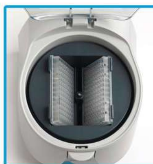
Before & after centrifugation (angled position)
