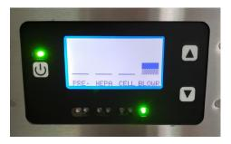
An advanced graphical display monitors the status of each filter and when they need to be replaced an LED lights up. A calibrated VOC/gas sensor is used to monitor filter effectiveness.
