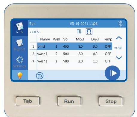
Touch screen control panel
