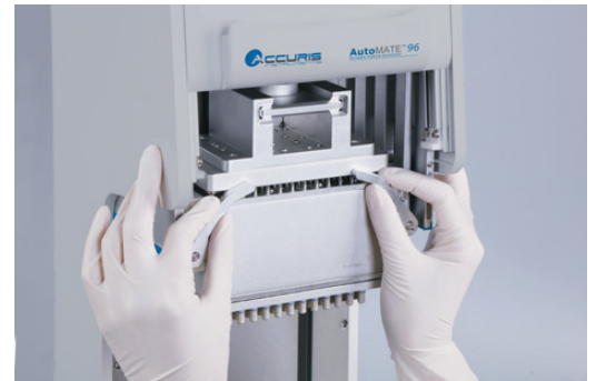
Easy Replacement of Pipetting Head
