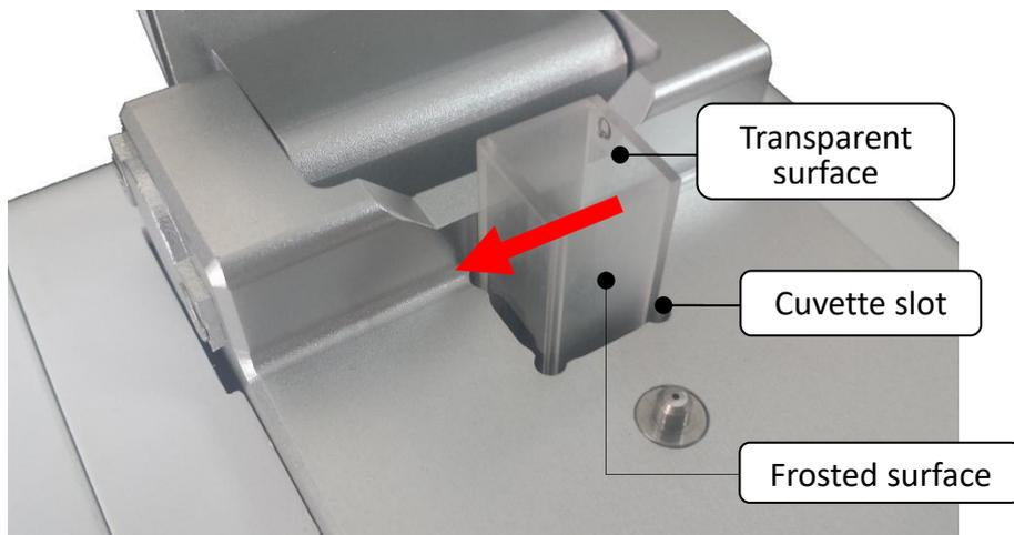
**Fig. 7 Cuvette Port**
