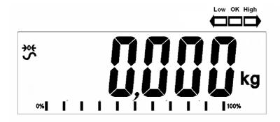
Place a container on the platform and a value for its weight will be displayed.  Press the [Z/T] key to tare the scale. The weight is deducted and stored as the tare value leaving zero on the display. The "NET" indicator will be ON and as a product is added only the net weight of the product will be shown. The scale could be tared a second time if another type of product was to be added to the first one. Again only the weight that is added after taring will be displayed.
