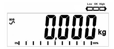
The scale has an automatic re-zeroing function to account for minor drifting or accumulation of material on the platform. However you may need to press the [Z/T] key to re zero the scale if small amounts of weight are shown when the platform is empty.
