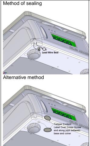
The scale has got metallic loops on the base and the cover, located at the right rear corner as shown here. A metal pin or wire can be passed through the loops and sealed using a lead-wire seal. Ensure the seal is secured enough to prevent removing the cover without breaking the seal or damaging the enclosure.
