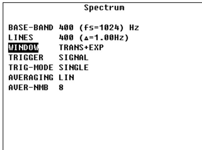
This is the standard setup screen for Spectrum measurement, which contains the same parameters as we need to define for frequency response function. See detailed description in [1], **Menu Dyn. Measur. – Setup menu → Spectrum Item** chapter. The new feature of this screen is the possibility to define several FFT window types.
