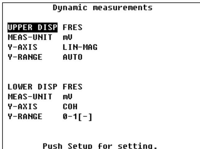
Set the both Dynamic measurement screens to FRES (frequency response function). The Dynamic measurement screen is used to set the upper display to LIN-MAG (linear scale) or LOG-MAG (logarithmic scale) and the lower display to COH (Coherence) or PHASE. The button **Info** works as the switch between all display modes.
