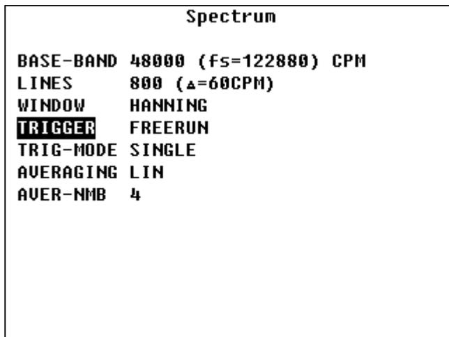
This screen is the standard setup screen for dynamic measurements ( *Dyn. Measur. – Setup menu – > Spectrum Item* ), see the [1], for detailed description. Return back to Dynamic measurement screen by pressing **ESC** . Run the measurement by pressing **START** . The result graph will have two forms.
