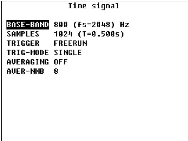
This screen is the standard setup screen for dynamic measurements ( *Dyn. Measur. – Setup menu – > Time Signal Item*), see the [1], for detailed description. Return back to Dynamic measurement screen by pressing **ESC** . Run the measurement by pressing **START**. The result graph will have two forms.
