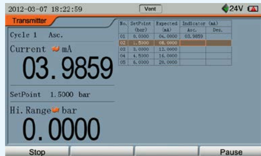
Pressure gauge / transmitter / switch calibration
