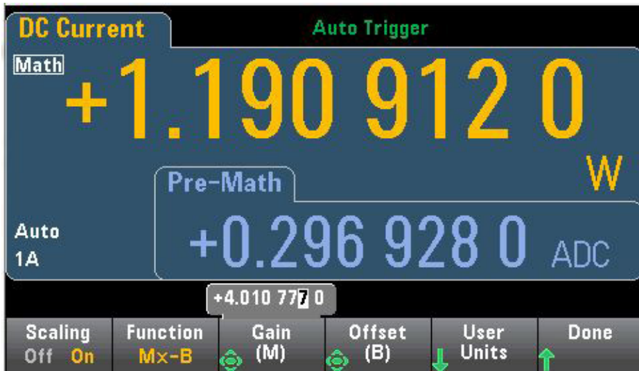
Figure 4. This screen displays the watt reading given the gain and raw current readings shown.
