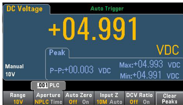
Figure 3. Peak measurement of DCV.
