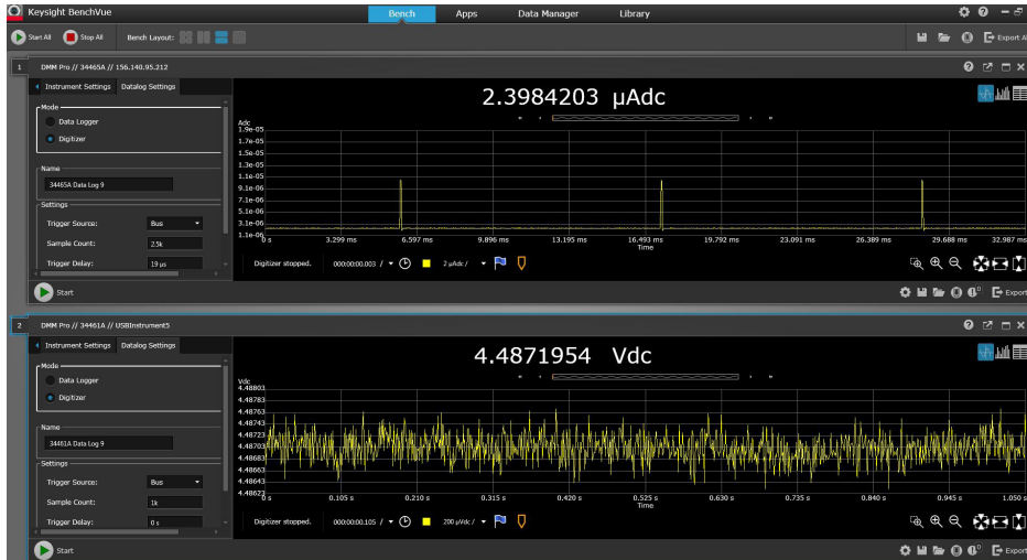
Figure 7. These two graphs illustrate the digitized DCI (top image) and DCV (bottom image) consumption.
