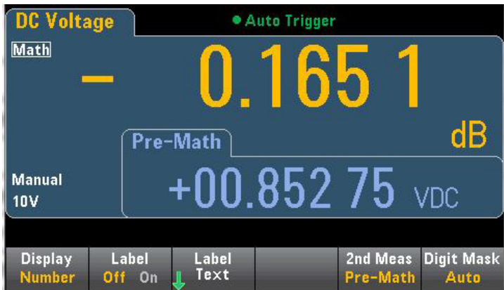
Figure 4. A DCV signal with dB scaling with the Pre-Math measurement.
