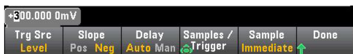
Figure 5. The Truevolt DMMs' advanced trigger modes allow designers to set a level trigger.
