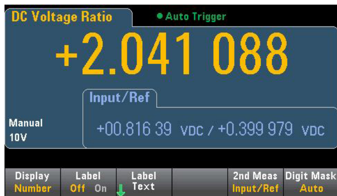
Figure 7. With the Truevolt DMM dual display, you can view 2 voltage measurements when using the DCV ratio function.
