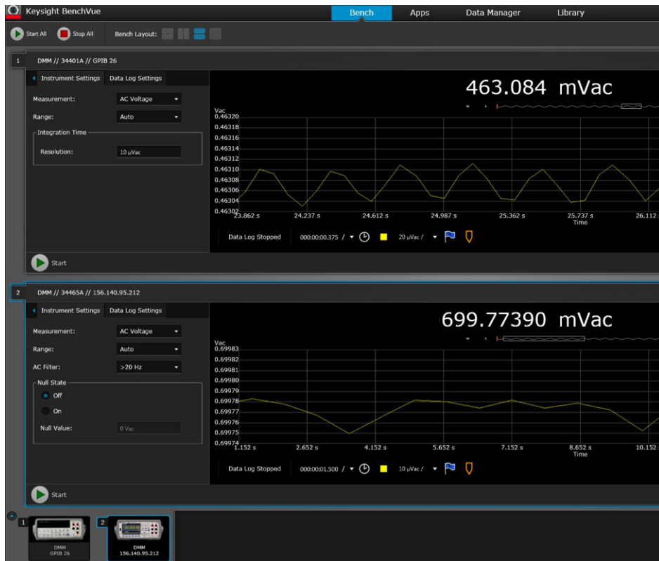
Figure 5. In this graphic, 1/10th of the V_{RMS} is measured accurately by the 34465A (bottom measurement).
