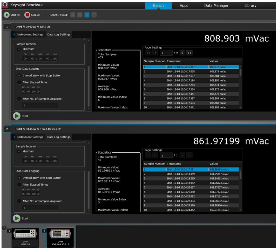
Figure 3. This display compares two parallel DMM readings. The reading taken with the 34465A DMM, at the bottom, measures the complete AC signal and hence, explains the higher reading value.
