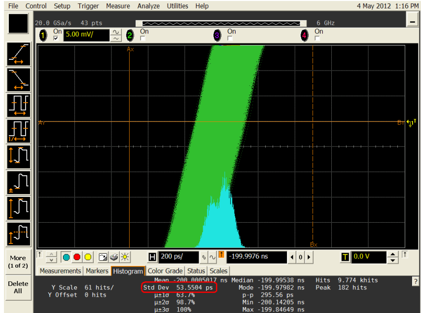
Figure 4. Jitter measurement on DDS signal
