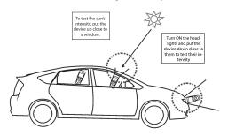
appear on the screen. Both the right and left headlights must be tested. Note the values and put them in your car for reference.
