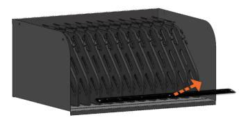
4 Pull forward, then up to remove the Divider.
