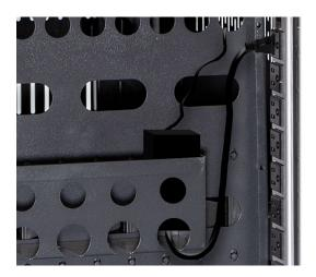
Working up front, weave device cables into divider tabs. Use supplied Cable Clips to fasten each cable to the divider by pressing down firmly.
