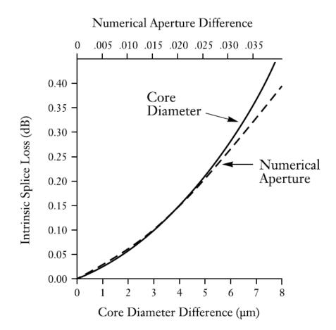
A core diameter mismatch of 5 microns can cause a 0.2dB loss.
