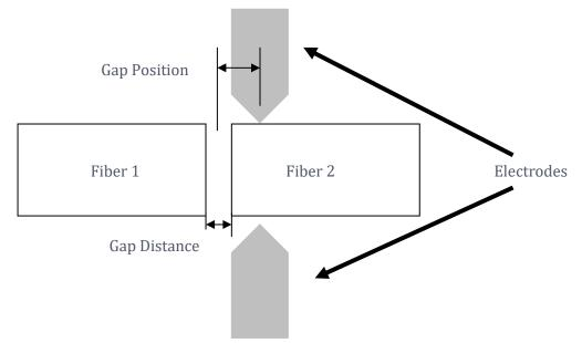
Fiber #1 melts easier so more energy is applied to Fiber #2.
