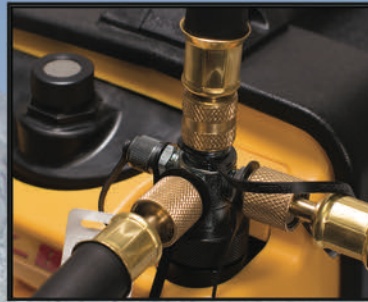
Use direct connections, large hoses, and no restrictions
