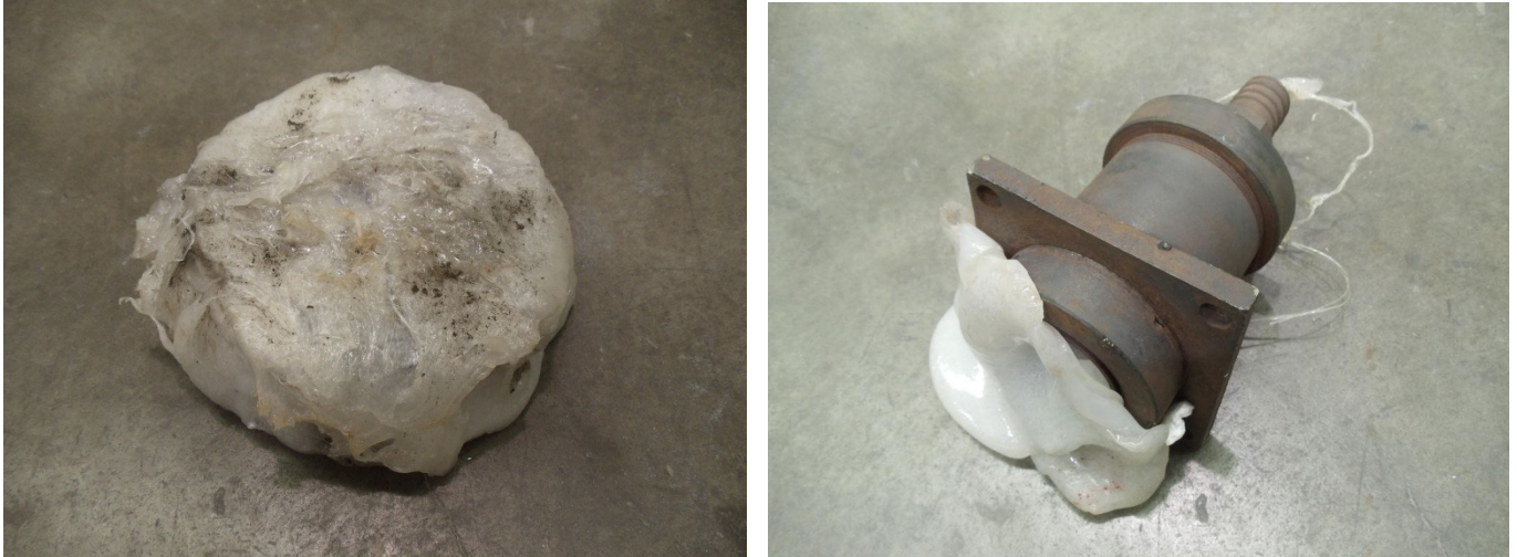
Fig.2 Pre-cleaning tool images. Left: breaker plate. Right: extrusion nozzle
