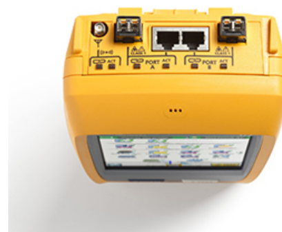
Figure 2: OneTouch™ AT connection ports
