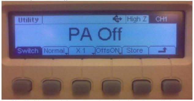
PA will be off by default, press the button corresponding with "Swtich" in order to enable the PA output. A output light will now be observed on the PA
