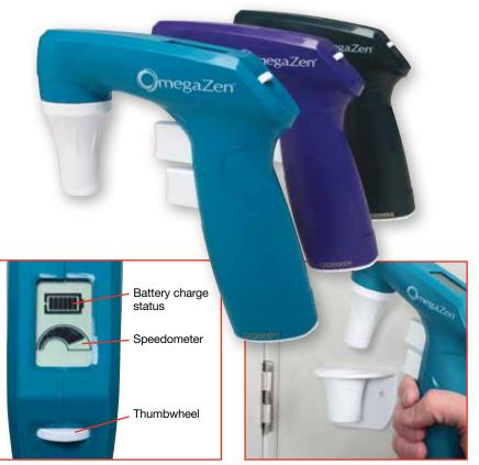
Turn thumbwheel and watch speedometer to fine-tune the speed.
