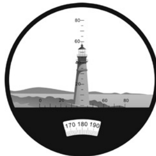
Figure 12. Vertical View Angle Measuring
