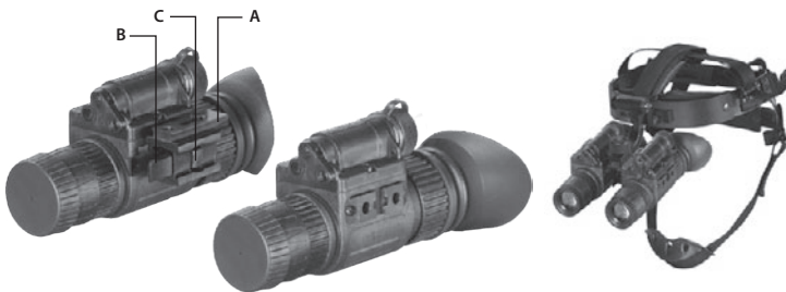
FIGURE 3-7. MOUNTING THE N-14 TO A DUAL BRIDGE
