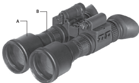
FIGURE 3-7. MOUNTING 3X AFOCAL LENSES TO THE N-15
