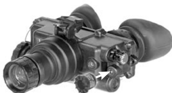
FIGURE 3-5. INSTALLATION OF THE IR SPOT/FLOOD LENS
