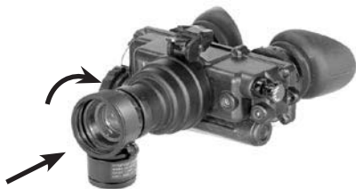
FIGURE 3-4. INSTALLATION OF COMPASS
