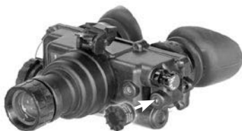
FIGURE 3-5. INSTALLATION OF THE IR SPOT/FLOOD LENS
