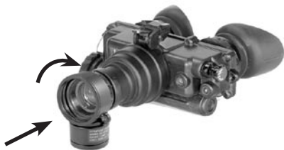
FIGURE 3-4. INSTALLATION OF COMPASS
