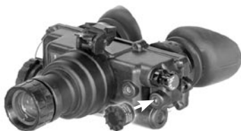
FIGURE 3-5. INSTALLATION OF THE IR SPOT/FLOOD LENS
