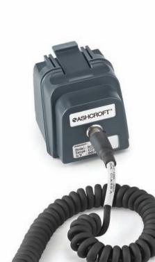
The Ashcroft ATE-2 provides accurate temperature measurement when using the AM2-RT module with an RTD probe. This system supports the most common RTD's without requiring operator input of probe characterization data; each module comes factory-programmed with standard curves for Pt100 (385 & 392), Ni 120, Cu 10 and temperature probes.
