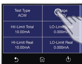
TAP TEST SETTING Tap the test parameter you would like to edit. Swipe up and down to scroll through test parameters.
